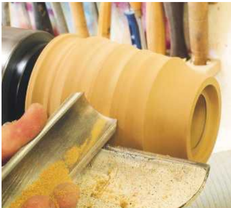
▲ Pic.7 Get the big guns out! The smaller Signature gouge was taking too long so Les went with the roughing gouge. Keep the flute pointing in the direction of the cut or it will dig in
